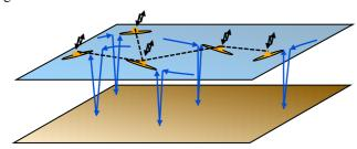
More precisely, in this framework, a team composed by a number n of AUV's that, when surfaced at a so-called k-th stage, are connected by a wireless network with given topology, are asked to perform (possibly in a synchronous way) a vertical dive and relevant re-emersion; during which the associated k-th stage sample measurements of an oceanic field variable  $\theta(x)$ , at the reached depth, are collected by each vehicle composing the team.
