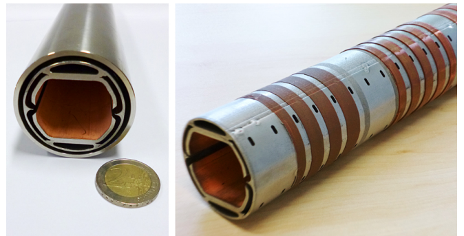
Figure 1. Prototype FCC-hh beam screen (courtesy of Cedric Garion and Javier Fernandez Topham – CERN).
