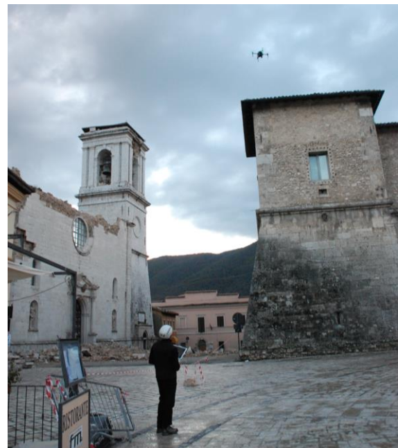
Figure 7. Photogrammetric survey with UAS.
