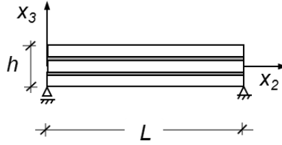
Figure 3: Simply supported wide plate with n layers and n-1 imperfect interfaces.
