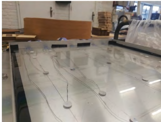
Fig. 11. Fully cured retrofit sensor layer.
