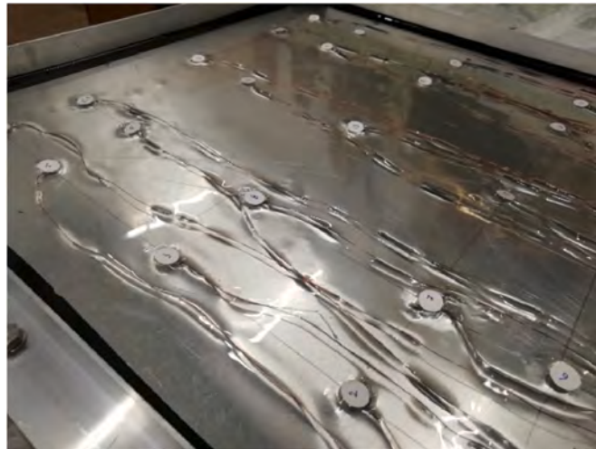
Fig. 10. Placing of the PZT sensors.
