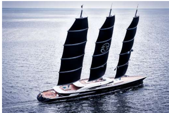
FIGURE 4.2: Oceanco Black Pearl rigged with DynaRig.[91]
