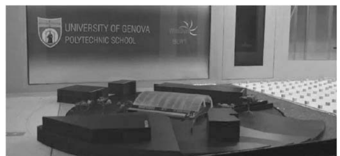
Fig. 6. Model on the turning table in the Giovanni Solari Wind Tunnel of the Genoa University.
