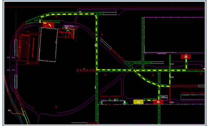
Figure 6: Underground path involving UGVs leading to the entrances of the three warehouses (red boxes).
