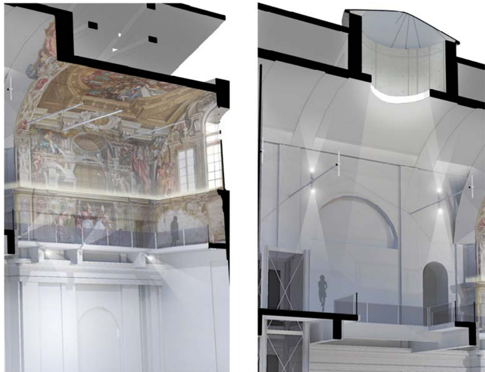
Figure 16. Detailed views of the walkway and lighting solutions for the sacred space of the church to be enhanced and returned to public use (elaboration of the students of the post-graduate programme, School of Specialisation in Architectural Heritage and Landscape).
