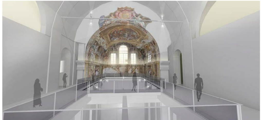
Figure 13. View of the new public space at the level of the former reading room and of the big “holes” in the reinforced concrete floor that allow to perceive, from the ground floor, the original holy space (elaboration of the students of the post-graduate programme, School of Specialisation in Architectural Heritage and Landscape).
