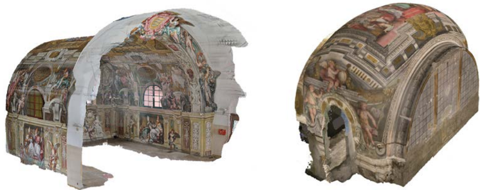
Figure 8. The survey in digital photogrammetry of the apse and a side chapel, still decorated (Gabriella Garello and students of the post-graduate programme, School of Specialisation in Architectural Heritage and Landscape).
