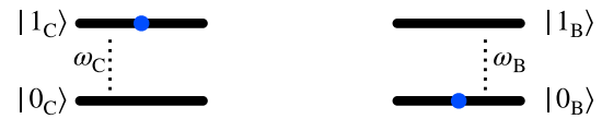
FIG. 1. Schematic representation of the two quantum systems. The first one, with energy separation \omega_C , acts as a charger (C), while the second, with energy separation \omega_B , can be seen as a QB (B).
