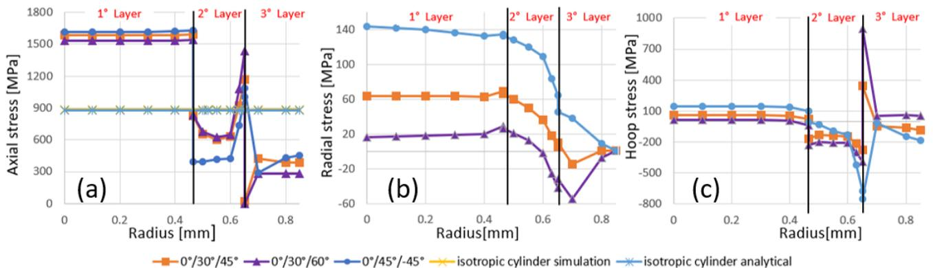
Fig. 4 – Stress distribution of Osteon A evaluated along a node path located in the mid-length of the model, in radial direction. (a) Axial stress in absolute value, (b) radial stress (c) hoop stress.
