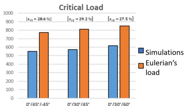
Fig. 5 – Comparison between the numerical and the analytical critical load
