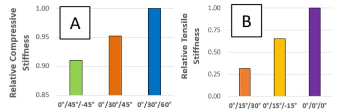
Fig. 3 – Uniaxial compressive (A) and tensile (B) results of OLSs. Simulation results are normalised with respect to the maximum value to allow a direct comparison in terms of compressive stiffness.
