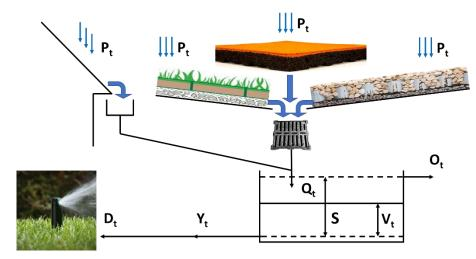
**Figure 2.** Schematics of the main elements of the simulated RWH system.  $P_t$  is the precipitation amount;  $Q_t$  is the rainwater inflow to the storage tank; *S* is the storage capacity of the system;  $V_t$  is the rainwater volume stored in the tank;  $Y_t$  is the released volume;  $O_t$  is the overflow volume; and  $D_t$  is the water demand.
