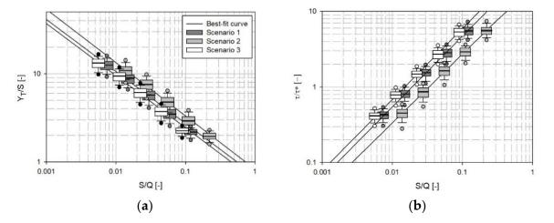
**Figure 5.** Box-and-whisker plots of the annual variability of the usage volume per unit of tank capacity ( $\mathbf{U} = Y_T/S$ , panel (**a**)) and normalized detention time ( $\tau/\tau^*$ , panel (**b**)) as a function of the storage fraction (S/Q) in the three investigated scenarios. The box-and-whisker description is the same as that in Figure 1. Continuous lines represent the power law regression function calculated from the annual mean values.
