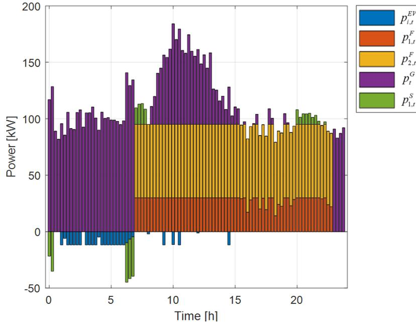
Fig. 4.5 Optimal microgrid scheduling
