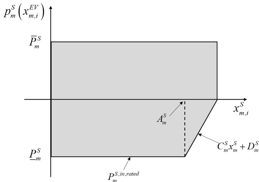
Fig. 5.9 Boundaries on the power exchange with the storage.
