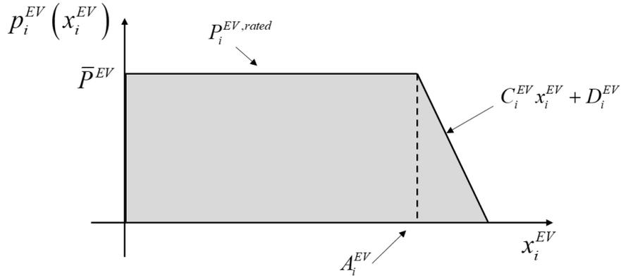
Fig. 5.4 Piecewise linear battery constraints (charging of EVs).
