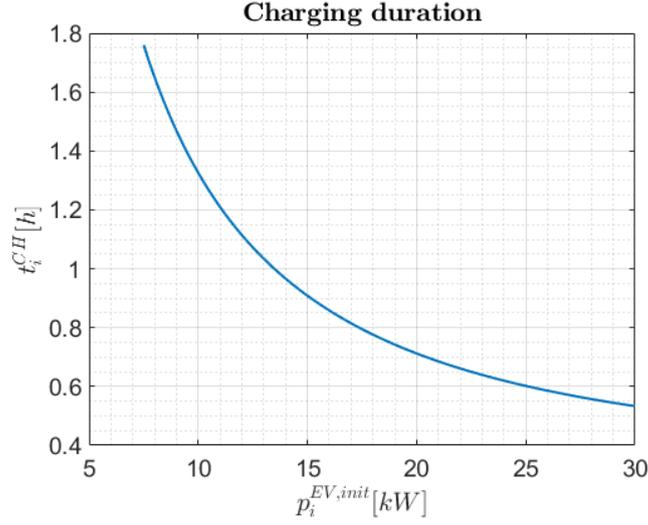
Fig. 5.7 Length of the charging interval according to the initial power.
