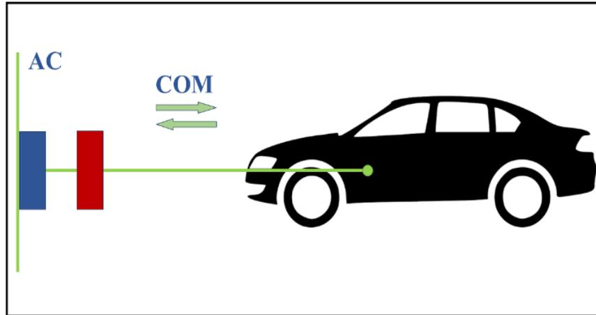
Fig. 2.4 Connection in "Mode 2" configuration.
