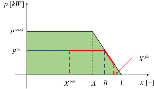
Fig. 6.2 The actual power profile of the battery (red line).
