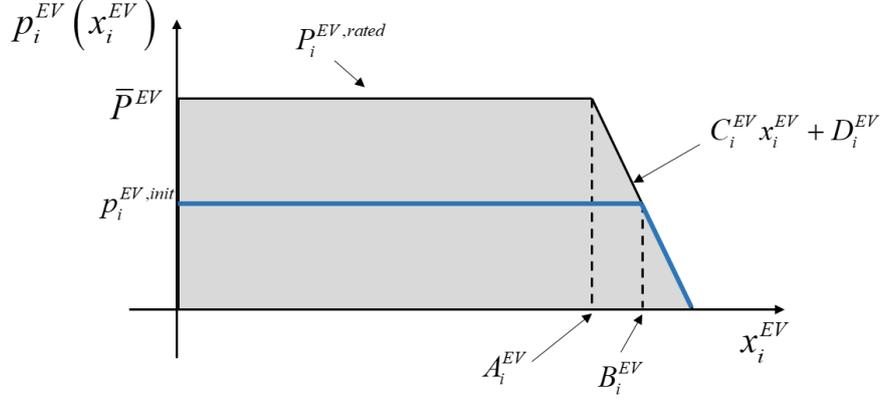
Fig. 5.5 The charging profile of the battery.
