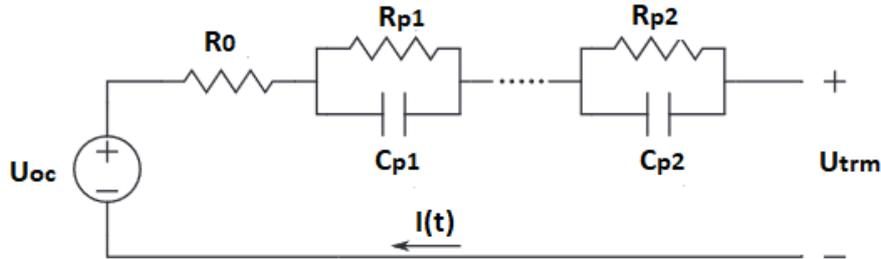
Fig 3.1 Dynamic RC battery model.
