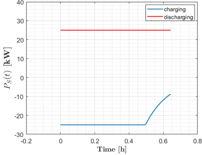
Fig. 5.10 Example of the charging (blue)/discharging (red) process of the storage.
