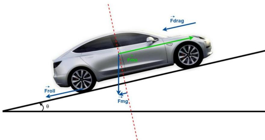
Fig 3.3 The forces of a vehicle in motion.
