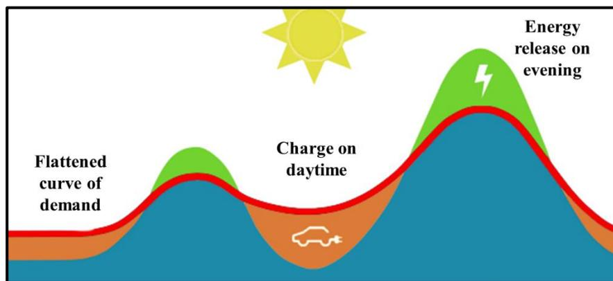
Fig. 2.12 Vehicle-to-Grid mechanism.
