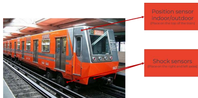
Fig. 3. Sensors installed by STIMIO.
