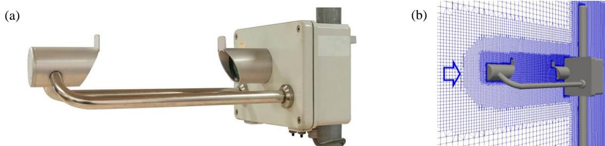
**Figure 1.** In panel (a) the Thies LPM, with the emitting head (attached to the circuitry box on the left-hand side) and the receiving head (attached to the supporting arms on the right-hand side). In panel (b) an example of computational mesh used.
