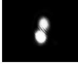
Figure 7.5: A picture of the pre-alignment procedure with the sub-carrier and the local oscillator beams on the Near-Field camera.
