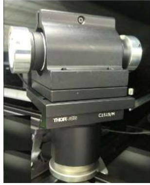
Figure 6.5: Piezo holder for fast CC loop. It is symmetrical and hosts two mirrors and two piezos. The idea is to push simultaneously the mount from both the side in order to mechanically dump the resonances.
