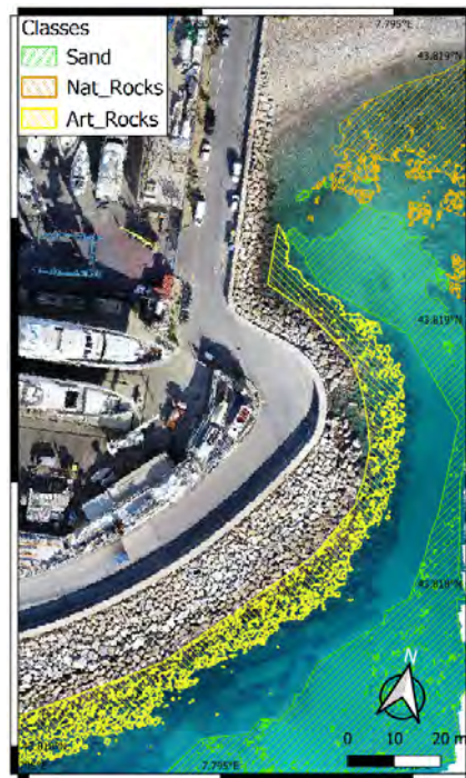
Figure 13. Seabed classification: areas with the same classes of seabed identified by the three classifiers, i.e., sandy areas (green), natural rocks (orange) and artificial rocks (yellow). The UAV-derived orthophoto is used as background. Portosole (beach area excerpt).
