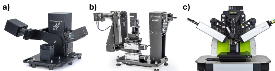
Figure 2.4: a) J.A. Woollam M2000 ® rotating compensator ellipsometer. b) J.A. Woollam VASE ® spectroscopic ellipsometer c) Nanofilm_ep4 from Accurion GmbH ® .
