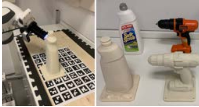
Figure 6.5 Left : the testing setup with the DIGIT sensor touching the “bleach cleanser” object. Right : example of YCB objects and their 3D printed counterparts.
