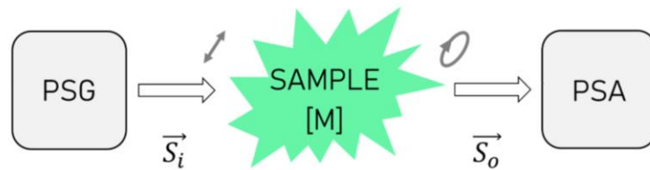
Figure 1 - The PSG stage generates the proper light polarization (grey double-sided arrow). The output polarization state is altered if the sample contains any anisotropy (grey ellipsoidal arrow). The PSA analyzes such alterations by projecting the intensities associated with different polarization components onto a pre-determined basis.
