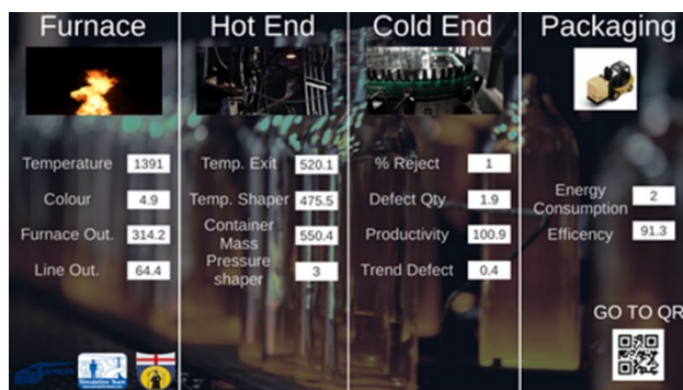
Figure 3. Mobile Dashboard for a glass production line.
