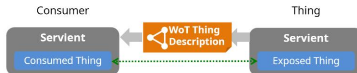
Figure 7. High-level architecture of Consumer – Thing interaction.
