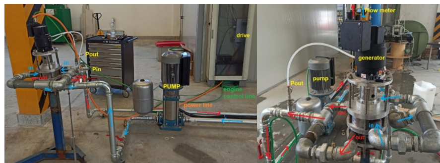
Fig. 4. Water expander experimental test rig
