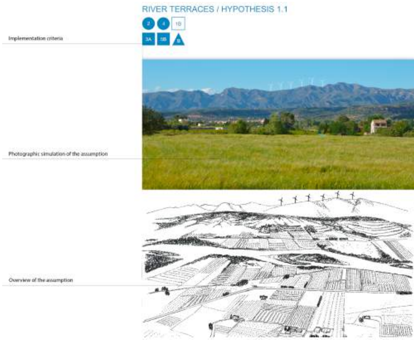
Figure 5. River terraces 1.1. Example of installation hypothesis in a representative scenario through the application of the identified criteria. Criteria adopted: 2: In general, wind turbines are arranged according to clear and regular geometric organizations (lines, curves, grids, etc.) and from the landscape patterns of the place to provide readability to the whole and reduce the feeling of clutter and visual confusion. 4: Spacing is regular between wind turbines and wind turbines of the same model, height, and color are used to emphasize the order and consistency of the set. 1B: The location of wind turbines on the last ridge line of a succession of reliefs substantially modifies a potentially unique characteristic and it has high visibility from medium distances. 3A: The linear arrangement of wind turbines in a wavy landscape following their morphological characteristics generates a clear and balanced image. 5B: It is important that the location and size of the wind turbines are consistent with the overall scenario and do not compromise the differentiated characters of the mountain and lowland agriculture. B: The implementation assumptions offer indicative heights for wind turbines from 50 m. (All images and photo-simulations in this article were taken from the document “Wind Energy and Landscape. Guidelines for a suitable installation in Catalonia”. They were drawn up by the research group).
