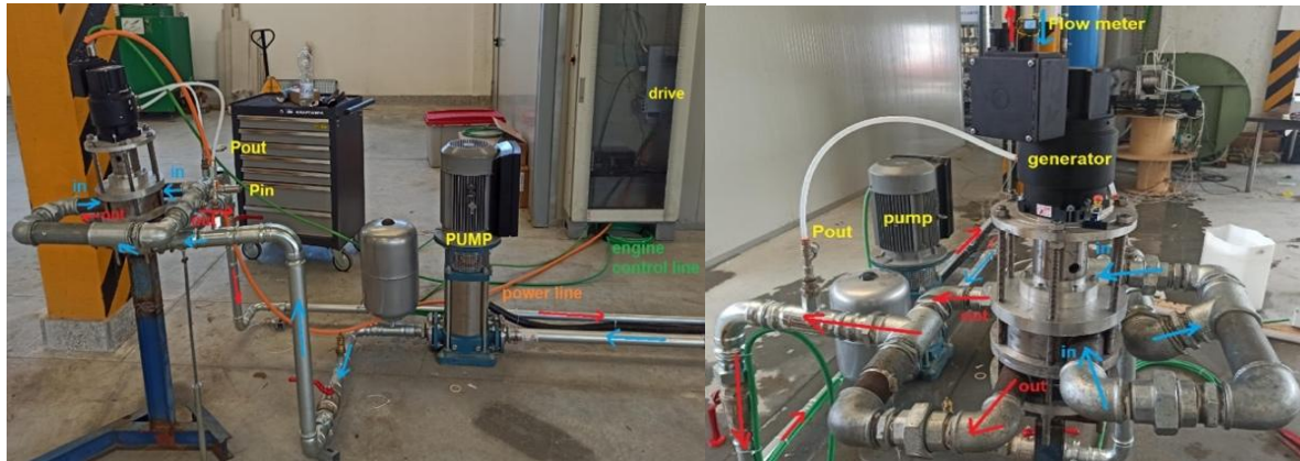
Figure 6 - Water expander experimental test rig
