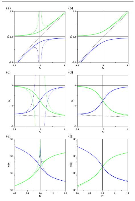
Fig. 8 The celerities  $(\mathbf{a}, \mathbf{b})$ , growth rates  $(\mathbf{c}, \mathbf{d})$  and relative amplitude of the free surface  $(\mathbf{e}, \mathbf{f})$  for (m2) (green solid line) and (m3) (blue solid line) exact eigenvalues compared with the outer  $(\mathbf{a}, \mathbf{c}, \mathbf{e})$  and the inner  $(\mathbf{b}, \mathbf{d}, \mathbf{f})$  approximate solutions (green and blue dashed lines)
