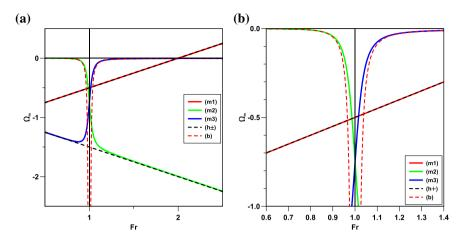
**Fig. 6** The growth rates (**a**) of the three eigenvalues of the morphodynamic problem; plot (**b**) is an enlargement of the transcritical ( $Fr \simeq 1$ ) region. The dashed black lines represent the growth rates of the two hydrodynamic eigenvalues (30) whereas the dashed red line represents the growth rate of the quasi-steady bed eigenvalue (43)
