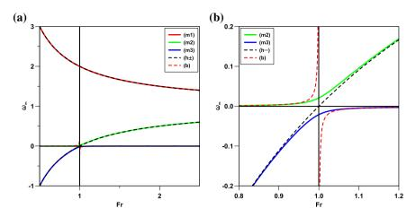
Fig. 5 The wave speed (a) of the three eigenvalues of the morphodynamic problem; plot (b) is an enlargement of the transcritical ( $Fr \simeq 1$ ) region. The dashed black lines represent the celerities of the two hydrodynamic eigenvalues (30) whereas the dashed red line represents the celerity of the quasi-steady bed eigenvalue (43)
