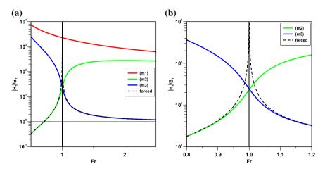
Fig. 7 The amplitude of the free surface associated with the three morphodynamic eigenvalues for a unitary bed amplitude (a); plot (b) is an enlargement of the transcritical ( $Fr \simeq 1$ ) region. The dashed black line represents the forced solution given by (39)
