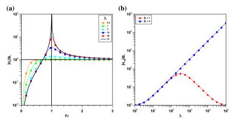
**Fig. 4** Amplitude of the free surface wave with respect to the bed wave: **a** as a function of the Froude number for several values of  $\lambda$ , for  $\delta_N=0$ ; **b** as a function of  $\lambda$  for Fr=1 (maximum amplitude), with  $(\delta_N=1)$  and without  $(\delta_N=0)$  the effect of the normal stress
