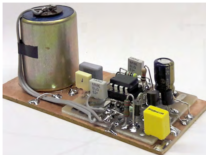
Figure 10. Picture of the geophone (left side) with an amplifier. Shielding and ground plane distribution were achieved using a copper board on which a second printed circuit board was located and electrically bonded where needed.
