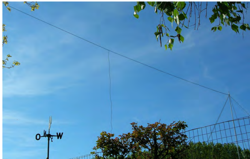
Figure 6. Picture of the Marconi wire antenna for E-field measurements (dimensions and construction details provided in the text).
