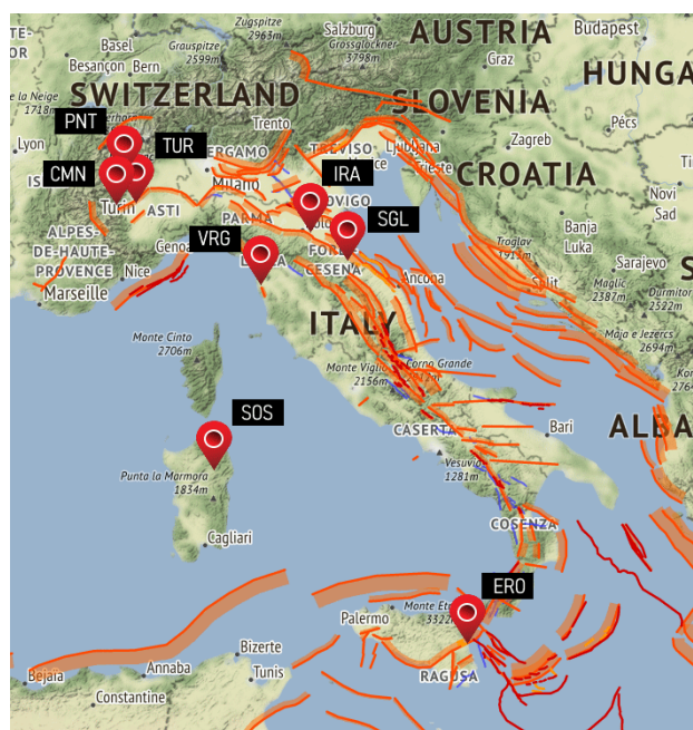
Figure 1. Location of monitoring stations over Italy: the six Opera 2015 stations are identified as CMN, PNT, TUR, IRA, SGL and ERO; the other two stations were added later, and they are SOS (for Sos Enattos in Sardinia) and VRG (for the EGO installation at Cascina near Pisa, in cooperation with the Virgo project).
