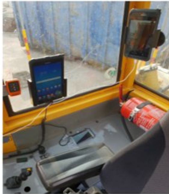
Fig. 6.8 Taking sensor measurements using Smartphones to classify the state of a Dumper in an earth-moving site (Axelsson and Wass (2019)).
