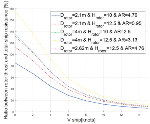
Figure 6. Influence of rotor geometry on rotor thrust.
