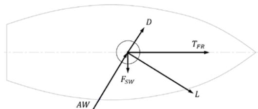
Figure 1. Rotor thrust from lift and drag.
