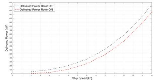
Figure 3. Delivered power ( $P_D$ ) with or without rotor.
