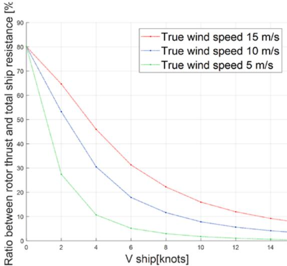
Figure 5. Influence of true wind speed on rotor thrust.
