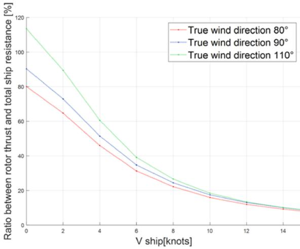
Figure 4. Influence of true wind direction on rotor thrust.
