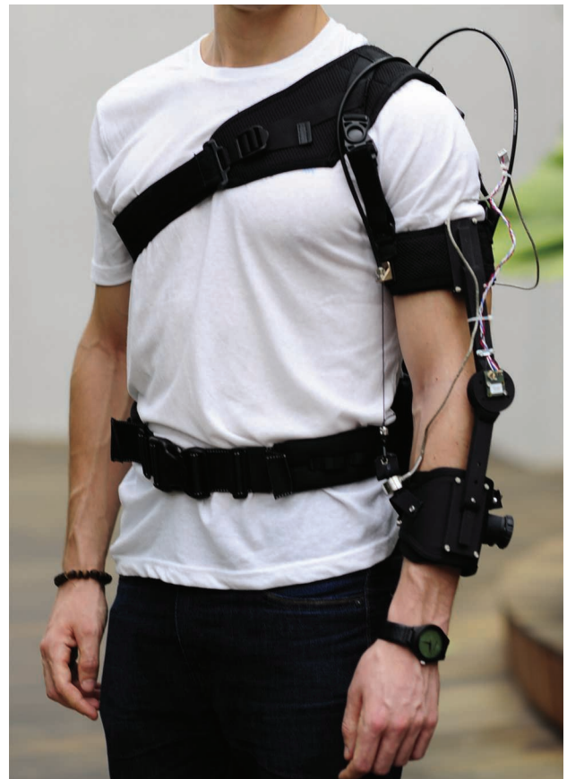
Figure 1. The exosuit device. The exosuit for elbow-joint assistance is composed of three fabric straps: one around the forearm (distal anchor point), one around the arm (proximal anchor point), and a shoulder harness connected to the arm strap via adjustable webbing bands. Buckles, Velcro straps, and a Boa lacing system enable the suit to be tightened. A pair of Bowden cables is attached to the front and back of the arm strap and transmits power from an actuation unit to the anchor points. The assistance is provided by recovering the front cable during elbow flexion. During elbow extension, the motor releases the cable.
