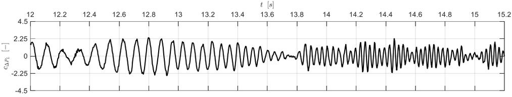
**Figure 2.** Time-history of  $c_{\Delta P_L}$  from one repeat of  $UF_1$ , focusing on the ramp-up.
