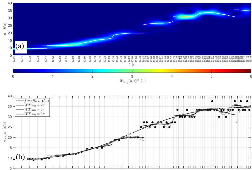
**Figure 3.** Time-frequency analyses carried out on the signal  $c_{\Delta PL}$  (Fig. 2): (a)  $\left|W_{c_{\Delta PL}}\right|^2$ ,  $\omega_0 = 6\pi$ , (b) variation of the shedding frequency in the transient.
