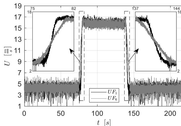
**Figure 1.** Comparison between the freestream velocity time histories of single repeats of UF<sub>1</sub> and UF<sub>6</sub>.
