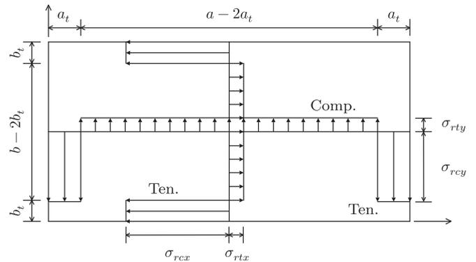
Fig. 7. Bi-axial distribution pattern of welding residual stress.
