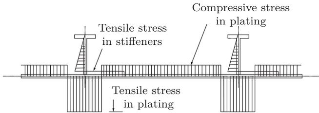
Fig. 5. Hybrid distribution pattern of welding residual stress.
