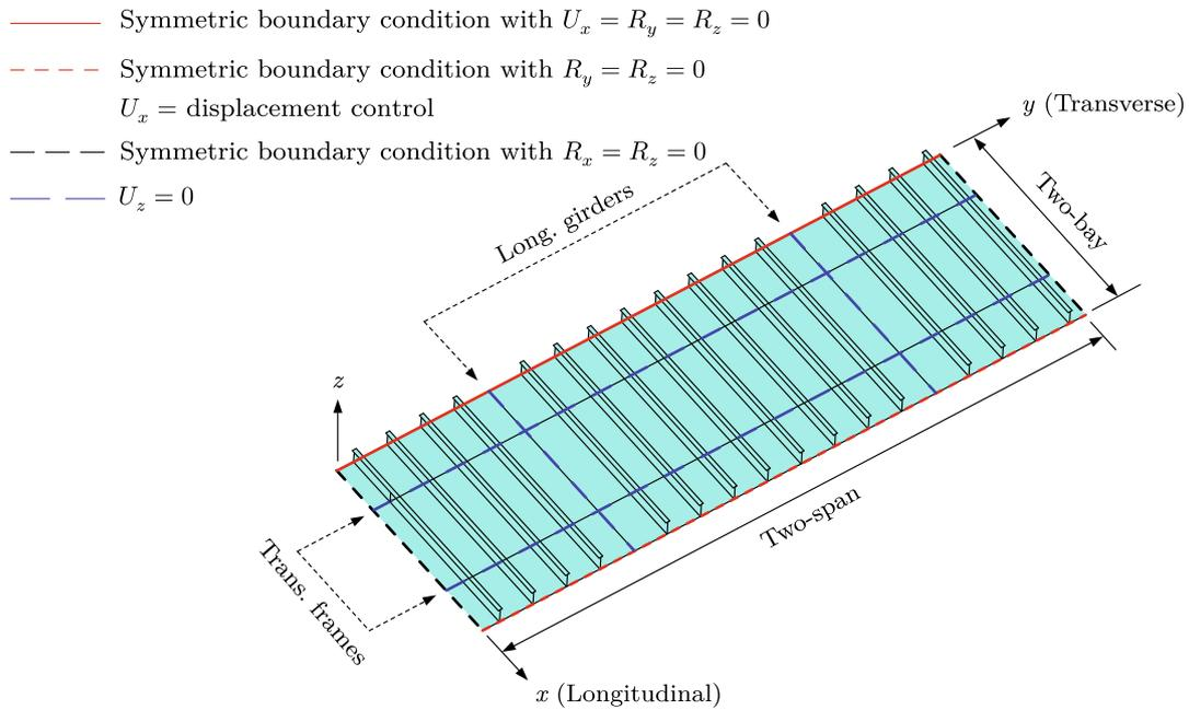
Fig. 2. Schematics of model extent and boundary condition.
