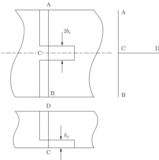
Fig. 6. Rectangular distribution pattern of welding residual stress.
