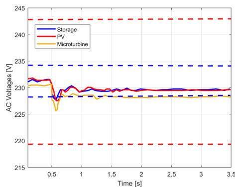
**Figure 8.** Simulation A: AC Voltages. The blue dashed lines represent  $V_{ac,ST,max}$  and  $V_{ac,ST,min}$ , while the red dashed lines represent  $V_{ac,PV,max}$  and  $V_{ac,PV,min}$ .
