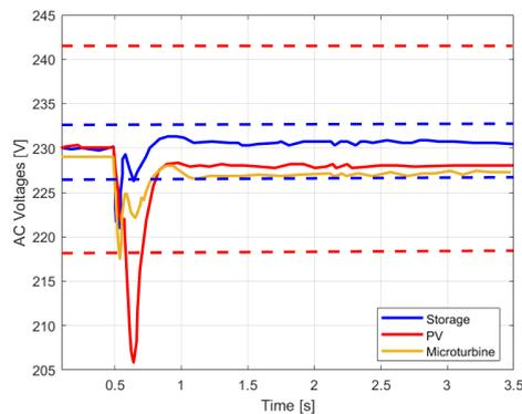
**Figure 11.** Simulation B: AC Voltages. The blue dashed lines represent  $V_{ac,ST,max}$  and  $V_{ac,ST,min}$ , while the red dashed lines represent  $V_{ac,PV,max}$  and  $V_{ac,PV,min}$ .
