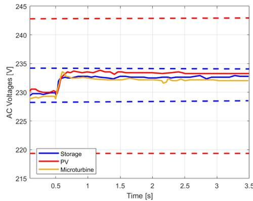
**Figure 14.** Simulation C: AC Voltages. The blue dashed lines represent  $V_{ac,ST,max}$  and  $V_{ac,ST,min}$ , while the red dashed lines represent  $V_{ac,PV,max}$  and  $V_{ac,PV,min}$ .
