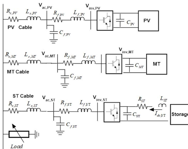
Figure 5. One-line diagram of test case MG.
