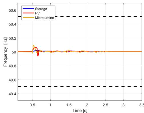
**Figure 15.** Simulation D: Frequencies. The dashed black lines represent the frequency limits  $f_{min}$  and  $f_{max}$ .
