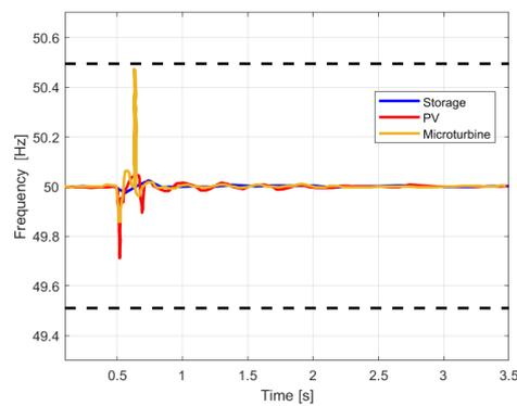
**Figure 6.** Simulation A: Frequencies. The dashed black lines represent the frequency limits  $f_{min}$  and  $f_{max}$ .
