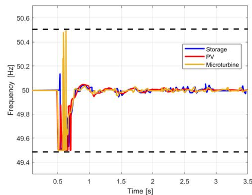
**Figure 9.** Simulation B: Frequencies. The dashed black lines represent the frequency limits  $f_{min}$  and  $f_{max}$ .
