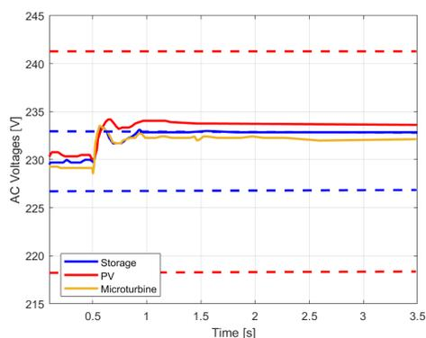
Figure 17. Simulation D: AC Voltages. The blue dashed lines represent  $V_{ac,ST,max}$  and  $V_{ac,ST,min}$  while the red dashed lines represent  $V_{ac,PV,max}$  and  $V_{ac,PV,min}$ .
