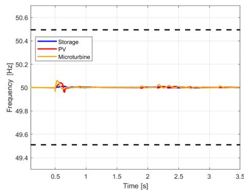
**Figure 12.** Simulation C: Frequencies. The dashed black lines represent the frequency limits  $f_{min}$  and  $f_{max}$ .
