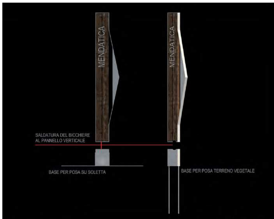
Figure 6. Technical drawing of the installation, featured with material and constructions details, applied on the single element
