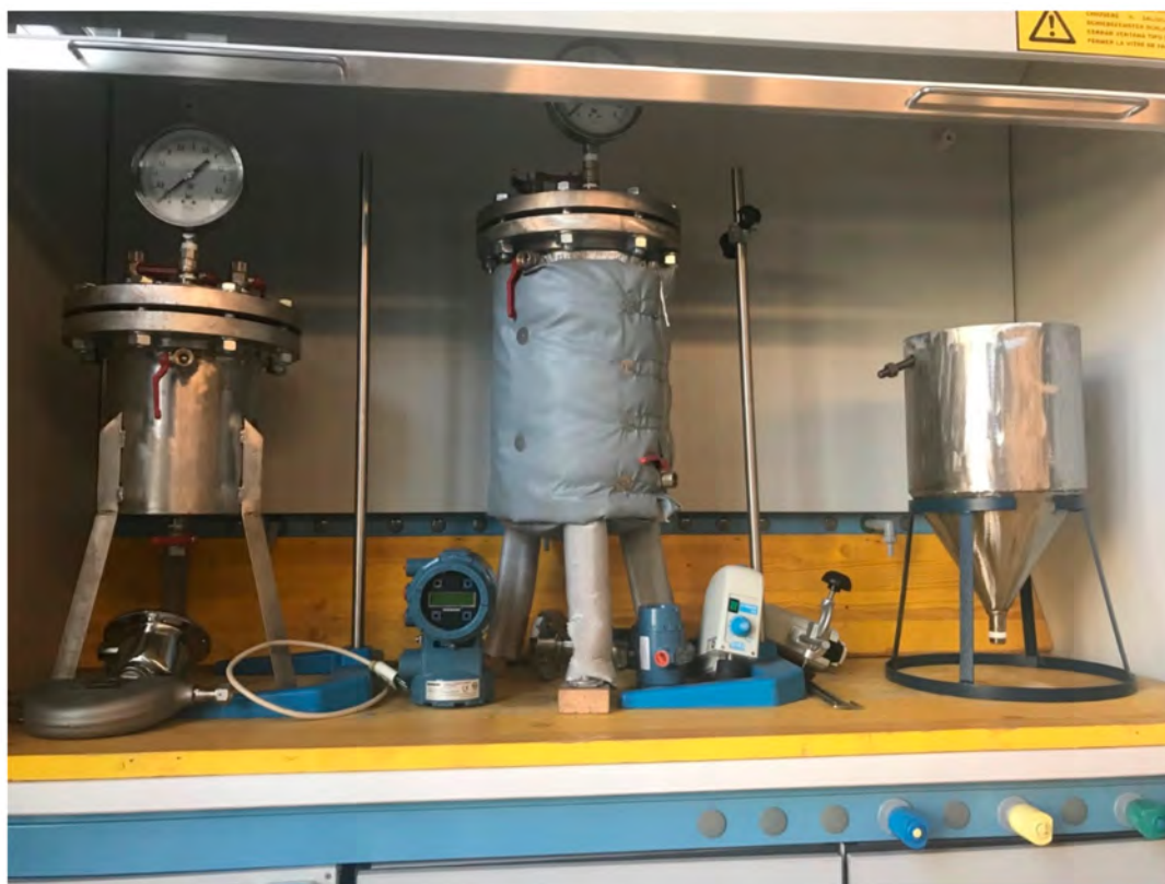
Figure 4. Pilot-scale biodiesel production. Mixer (left), transesterification reactor (center), decanter (right).
