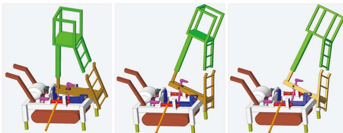
Fig. 3 Different orientations of the ladder with the cradle mechanism
