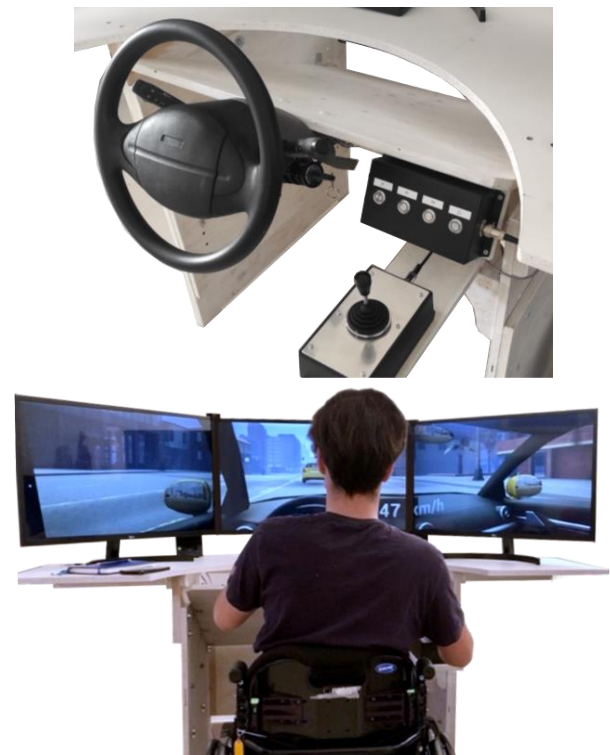
Figure 1. Hardware components of ADRIS 3.0. Real car steering wheel, automatic transmission and adapted brake/accelerator (top), and the three-screen configuration for improving the driving experience (bottom).
