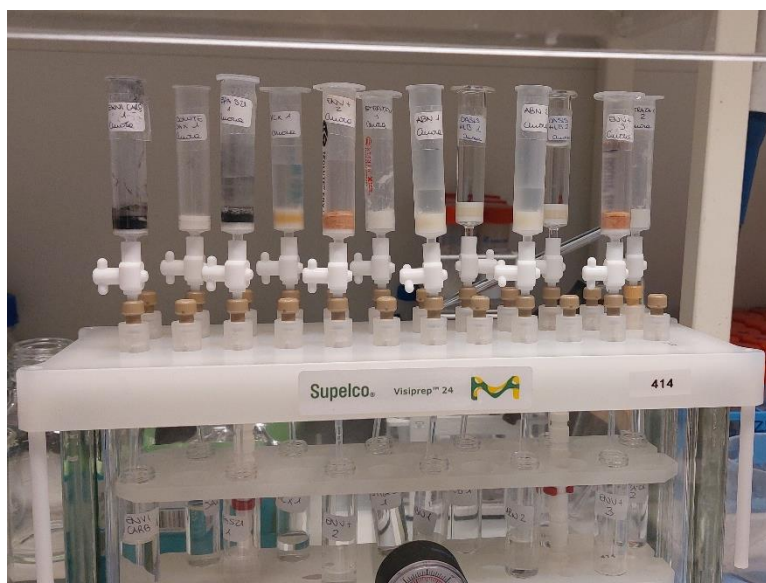
Fig. 7.4 Cartridges employed for the evaluation of their sorption ability towards nitramines.
