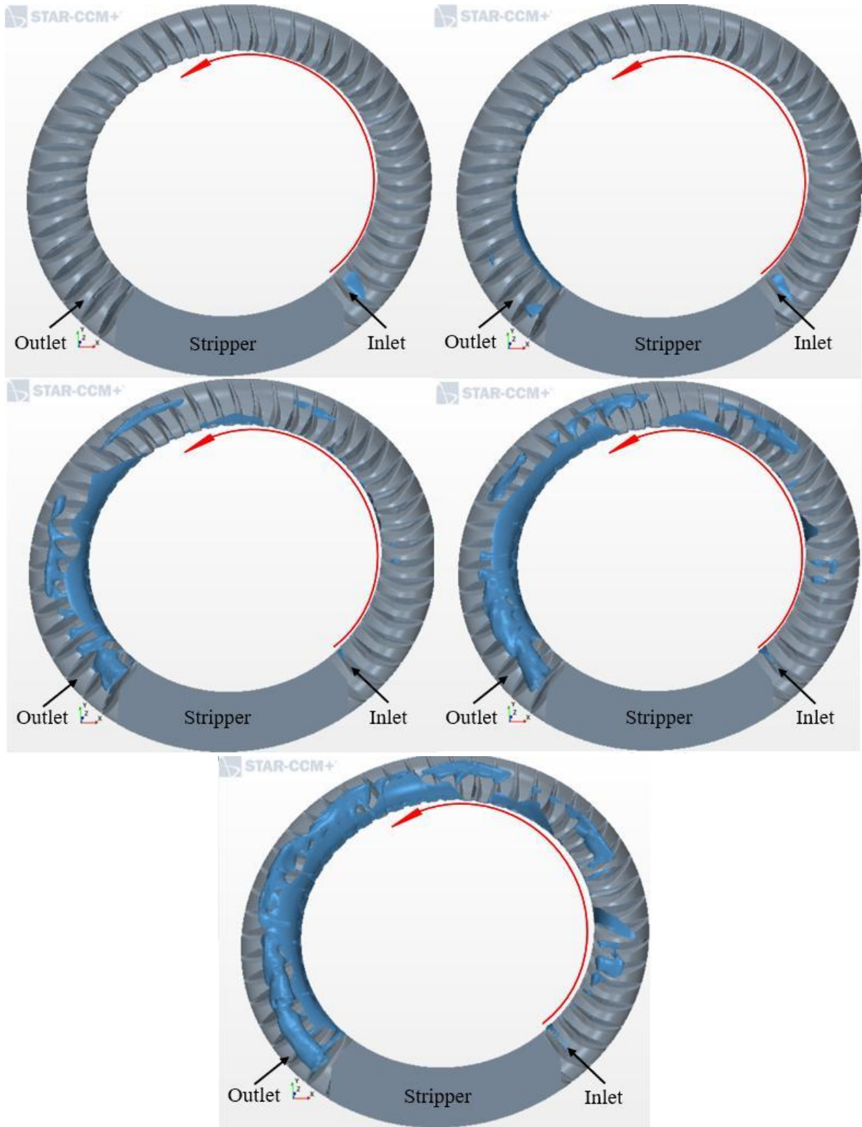
Fig. 40. separation zone in five working points at 3500 rotational speed.
