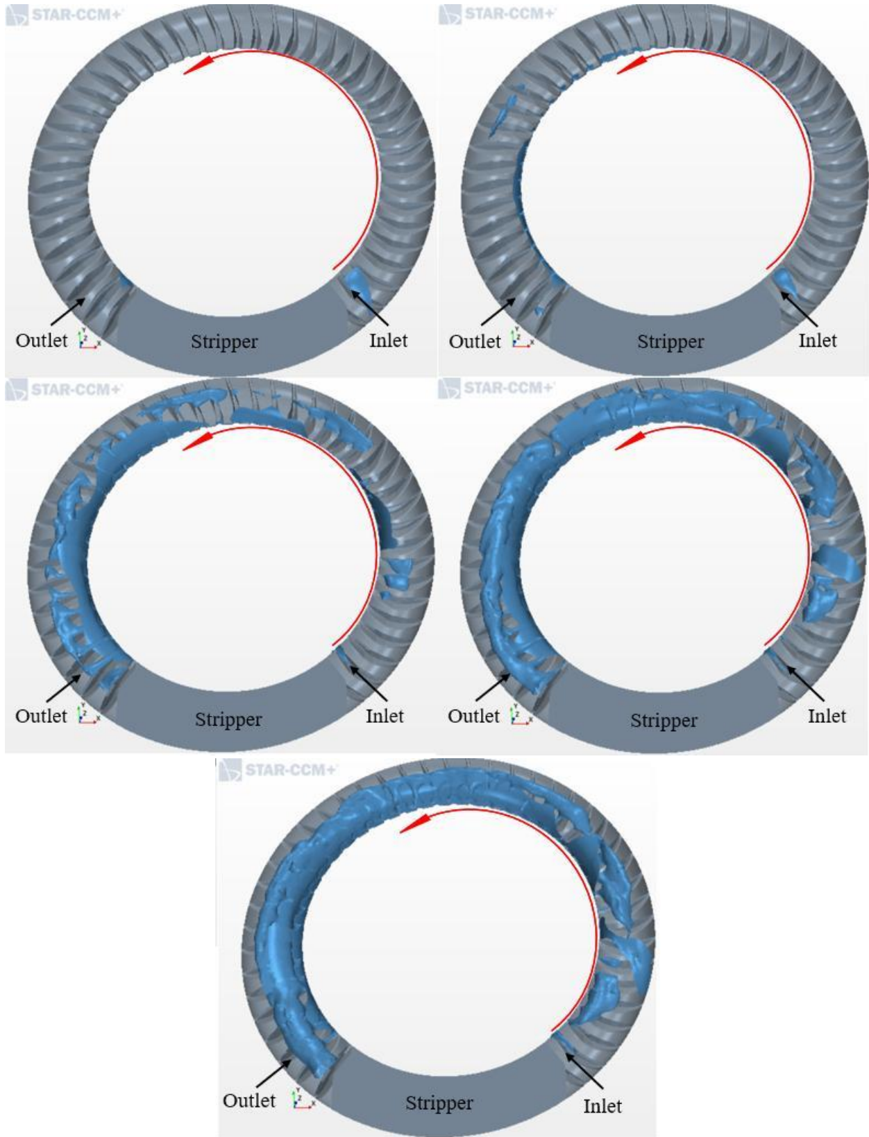
Fig. 44. separation zone in five working points at 2000 rotational speed.
