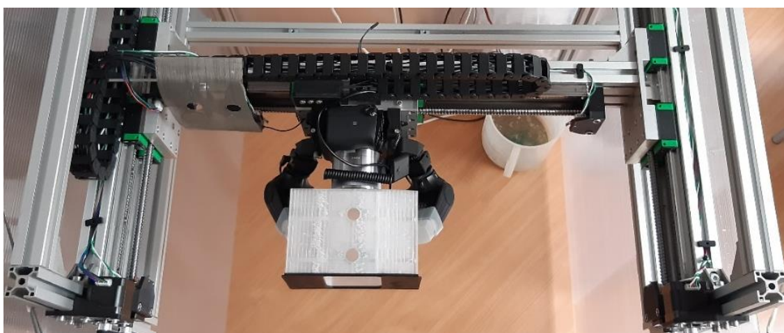
Figure 3: Picture of the PVS, with the camera, the two flashes and the diffuser.
