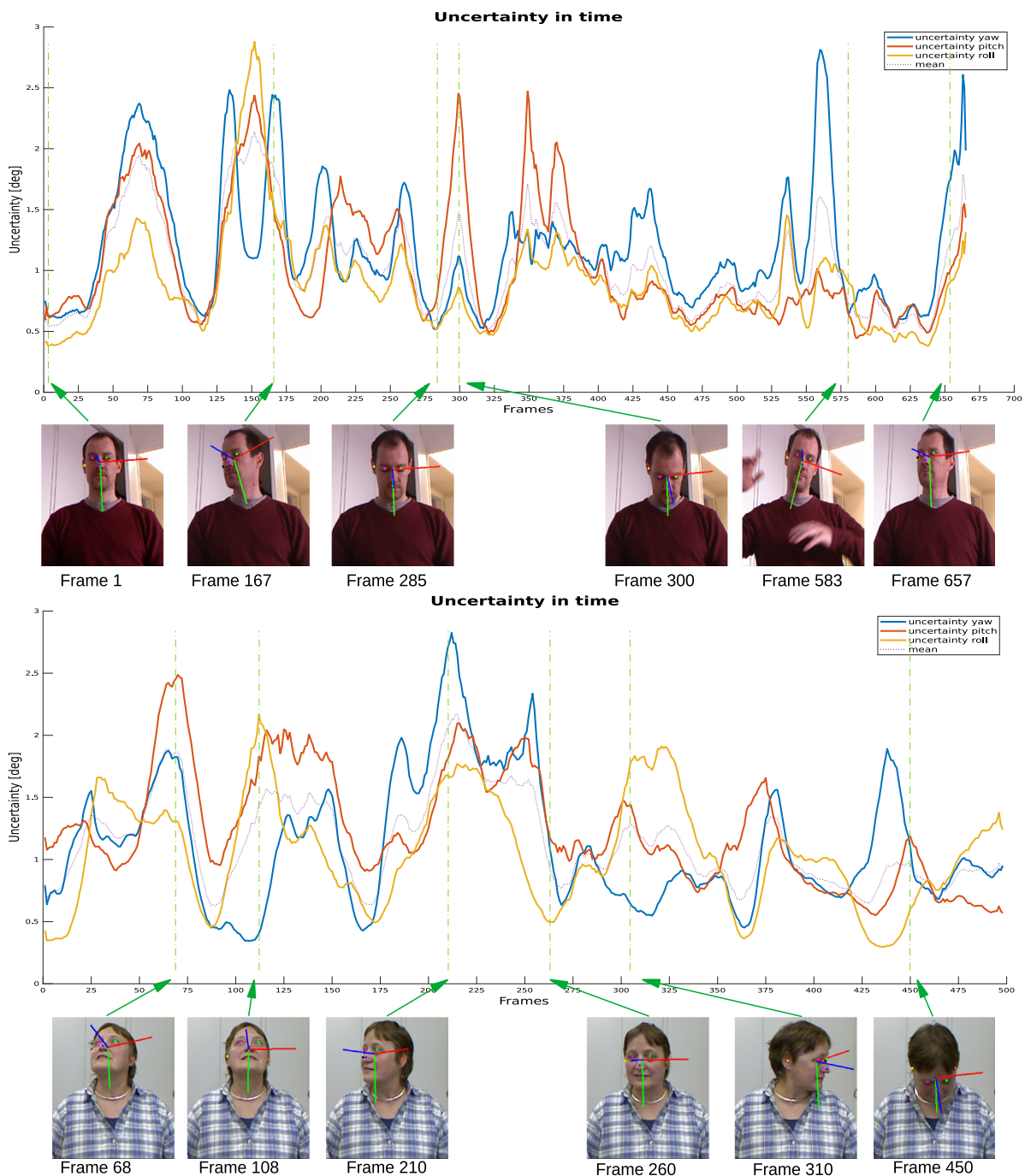
Fig. 6. Examples of how the uncertainties (in degrees) are influenced by the instantaneous head pose of a subject moving in front of a camera over time. We report in blue the yaw uncertainty, in orange the pitch uncertainty and in yellow the roll uncertainty. In dotted-purple we mark the mean uncertainty. The scale is in degrees of uncertainty. It can be observed that the uncertainties are very close to zero for the neutral head pose (frame 1 of the first sequence) and start to increase when the head rotates. (For interpretation of the references to colour in this figure legend, the reader is referred to the web version of this article.)
