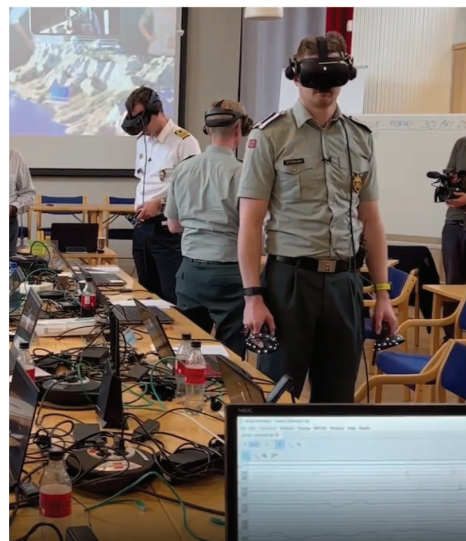
Figure 2: Example of an experimental session. Subjects are equipped with both the VR headset and EDA and PPG sensors.
