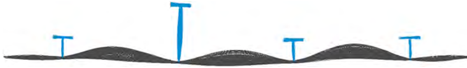
Fig. 11. Example of the measured imperfections applied to the FE model (plate and longitudinal stiffeners, values magnified by a factor of 10 for clarity).
