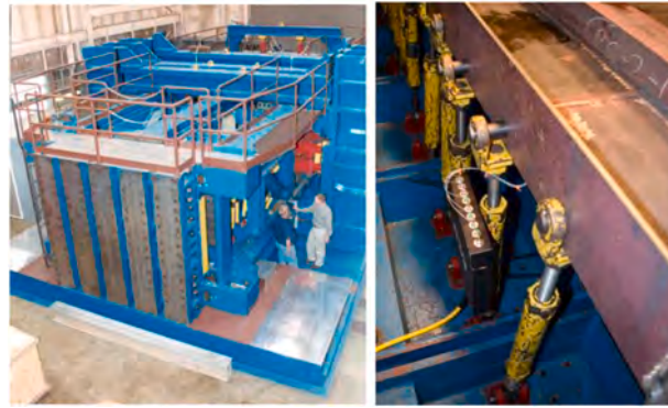
Fig. 6. (Left) Test fixture of the stiffened plate structure and (right) detailed view of the tie-downs and connection to the structure.
