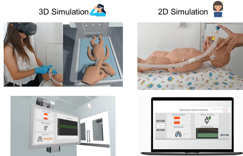
Fig 3. 2D and 3D simulation. Left: 3D simulation. The user wears the HMD and is immersed into a virtual environment showing a virtual representation of the manikin. Thanks to an HTC controller that tracks the neonatal island position, the virtual and real manikins are overlapped to each other and move accordingly. Right: 2D simulation. The user can physically interact with the manikin and receives feedback from a User Interface (UI) displayed on a computer screen. Sensors in the manikin and the face mask send data to the immersive VR application or the GUI to monitor the user performance in real time. UI description: Top left: the UI provides feedback about the manikin's head position. Top right: mask position; simple controls have been implemented to manage the colour code; if the area turns green, correct positioning; if the mask turns yellow, partially incorrect positioning; if the area turns red, completely incorrect positioning. Bottom left: Ventilation rhythm. If the sensor in the face mask is pressed (inhalation), the lungs in the UI are filled, during exhalation phase (sensor not touched), they are empty. Bottom right: chest compressions are shown on a line chart according to the data measured by the infrared sensor.
