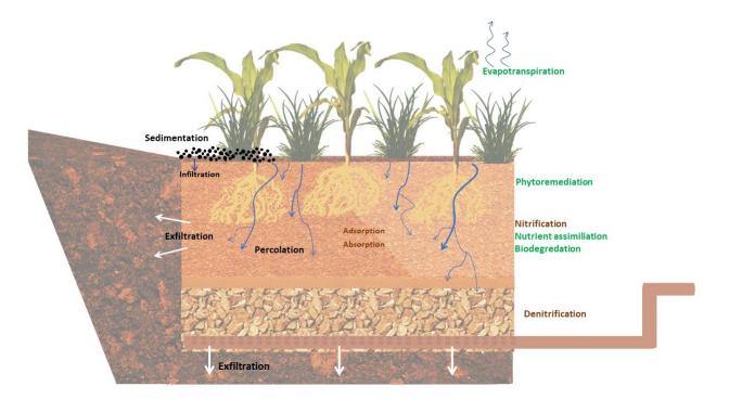
**Figure 3.** Fundamental physical (black label), biochemical/chemical (brown label), and biological (green label) mechanisms that occur in BRCs. Infiltration/percolation (blue arrows) and exfiltration (white arrows) are illustrated.
