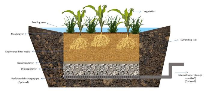
Figure 1. Schematic representation of a bioretention cell.
