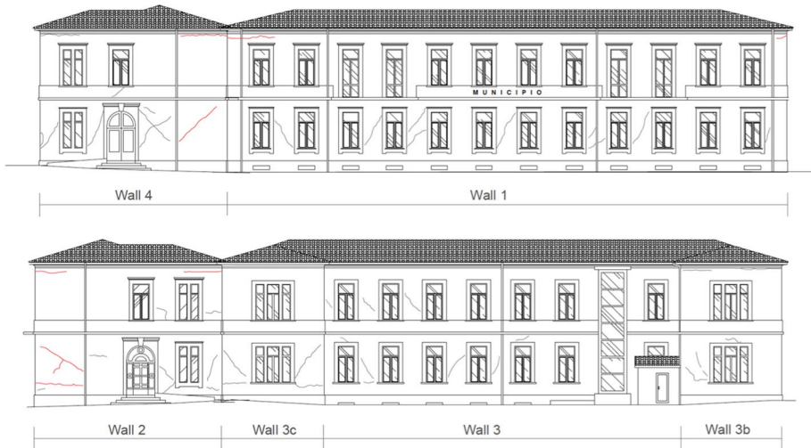
Fig. 2 Damage survey detected on the Pizzoli's town hall during the in-situ inspections performed after the mainshock of 18/01/2017—figure adapted from Degli Abbati et al. 2022 (local severe damage is in red)
