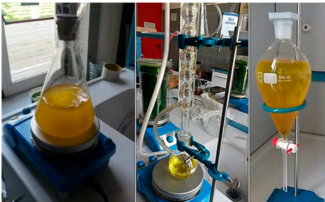
Figure 3. Lab-scale biodiesel production. Waste oil ( left ), catalyst and alcohol ( center ), decanter ( right ).
