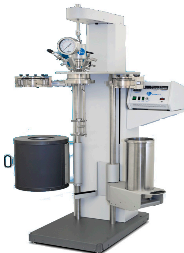
Figure 1. Photograph of the batch reactor used for p-cresol oxidation experiments.
