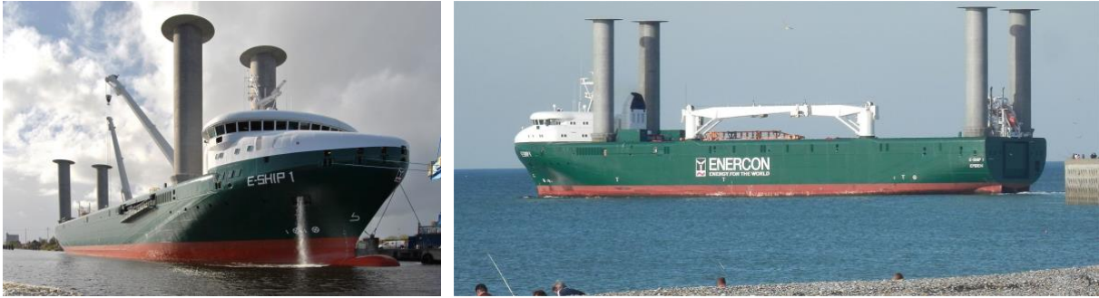
On the left: The E-Ship 1 with Flettner rotors at Emden; on the right: wind turbine transport vessel Enercon departing the Port of Dieppe on 24 September 2016.
