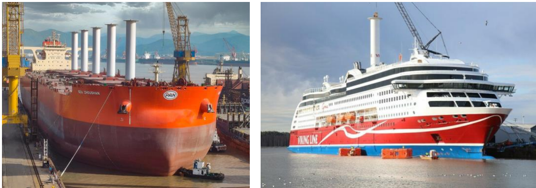
On the left: The M/V Sea Zhoushan of Brazilian mining company Vale, in Zhoushan, China on April 29, 2021, with five rotor sails installed along the vessel to allow for better efficiency; on the right: M/S Viking Grace , 57,565 gross tonnage ferry. The rotor is 24m high and 4m in diameter and is a modernized version of the rotor invented by Flettner. The rotor is controlled by a computerized system which detects the wind speed and puts it into operation automatically.
