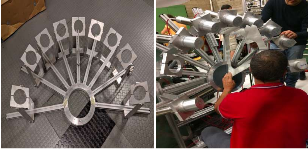
Fig. 5.13 On the left : the support structure to place the detectors at different \varphi_{LSci} angles. On the right : the LScis mounted on the "wheel".
