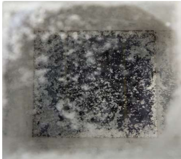
Fig. 5.3 TPB degradation on the acrylic windows. Whitish fragments were spread all around after the first warm up of the system, some can be seen deposited on the grid.
