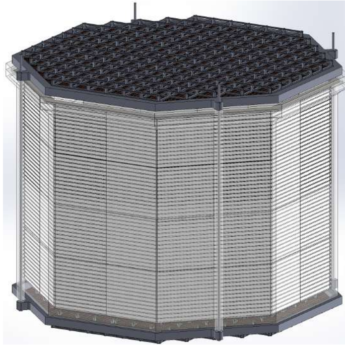
Fig. 3.7 DarkSide-20k octagonal TPC. An ultra-pure acrylic sealed structure will contain the ultra-pure underground argon used as active target. Just above and below the windows there will be the SiPMs arrays, held by special mechanical supports.
