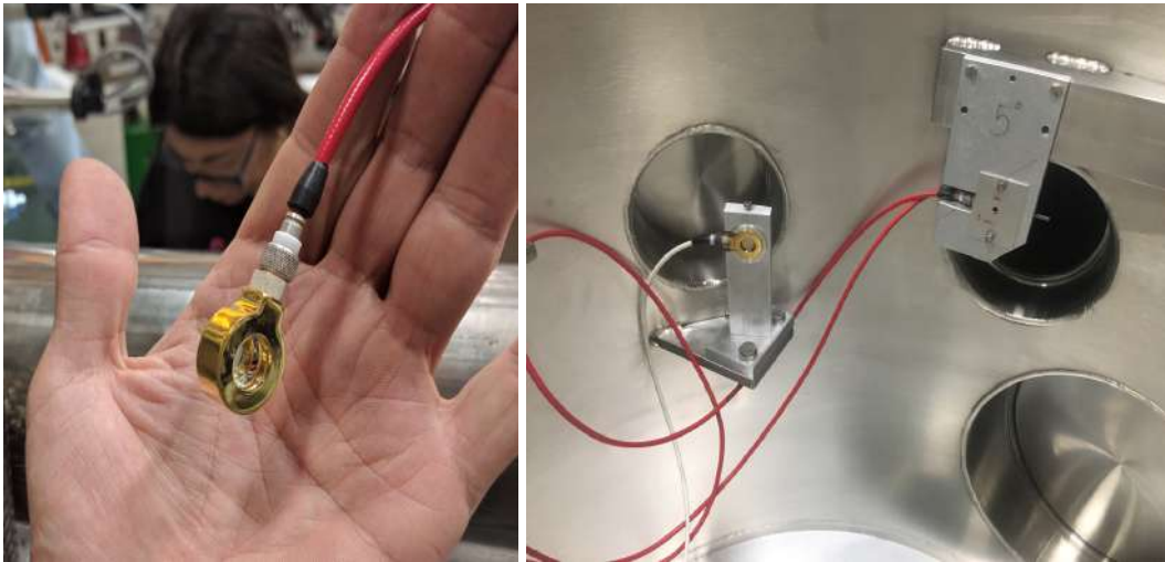
Fig. 5.11 Silicon telescopes in the scattering chamber
